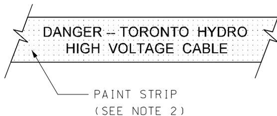
**DUCT IDENTIFICATION IN GROUND LEVEL FLOOR
