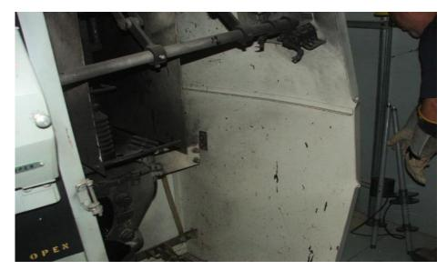
Figure 17: Impact of Internal Arc Fault in a Switchgear
